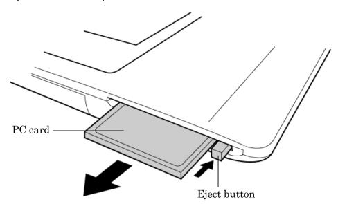
Figure 4-2 Removing the PC card
